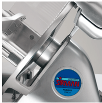
Remarkable clearance between blade and machine body
